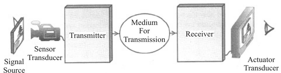
**Fig. 30.1** : A schematic arrangement for the communication system.
