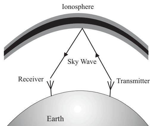
Fig. 30.9: Skywave propagation
