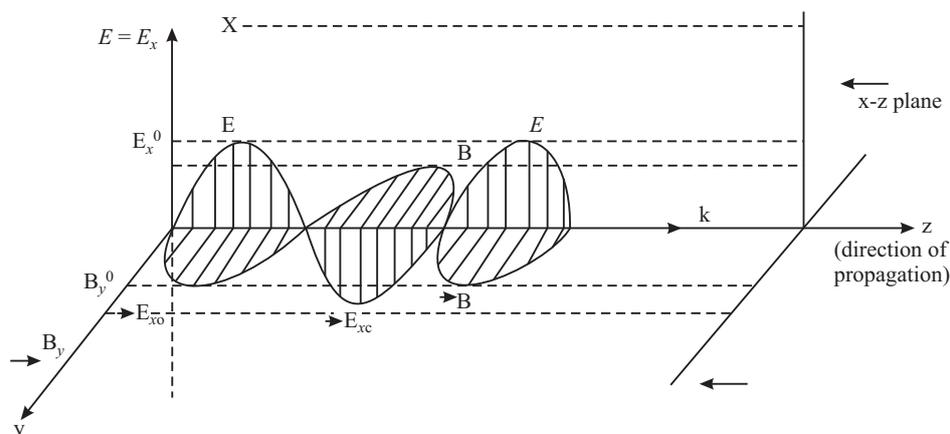
Fig. 30. 3: Propagation of electromagnetic waves
