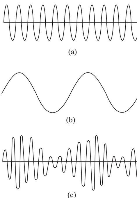
**Fig. 30.12:** Modulation of a carrier wave by a modulating signal: (a) a sinusoidal carrier wave of high frequency, (b) a modulating signal (message or information signal) of low frequency, (c) amplitude modulated carrier wave.
